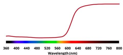
It is obvious to see from 600nm, which is just the start of red color in the visible spectrum, the TCS-9 spectral reflectance raises sharply, in consequence, if the light source does not have sufficient spectral power distribution in 600nm-800nm, it will be difficult to get a high R9. The capability of rendering the red color cannot be promised if the red spectrum is
